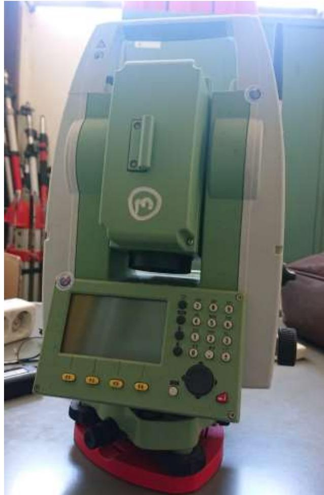
Gambar 3. 5 Inspeksi Total Station Leica TS-06
