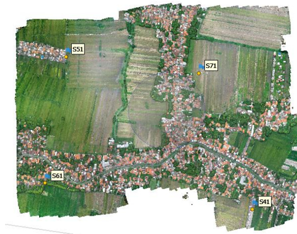
Gambar III.9. Hasil Proses Build Dense Cloud
