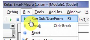
The image shows a screenshot of the Microsoft Excel VBA IDE. The title bar reads 'Kelas Excel-Macro 1.xlsm - [Module1 (Code)]'. The menu bar includes 'Debug', 'Run', 'Tools', 'Add-Ins', 'Window', and 'Help'. The 'Run' menu is open, showing options: 'Run Sub/UserForm F5', 'Break Ctrl+Break', and 'Reset'. A yellow circle highlights the 'Run Sub/UserForm F5' option, with a mouse cursor pointing at it. The background shows a portion of the VBA code editor with a line of code starting with 'Ln 7, C'.
