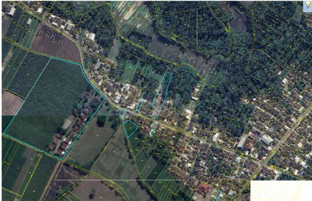
Keterangan Gambar : Hasil pembenahan peta no gap no overlap
